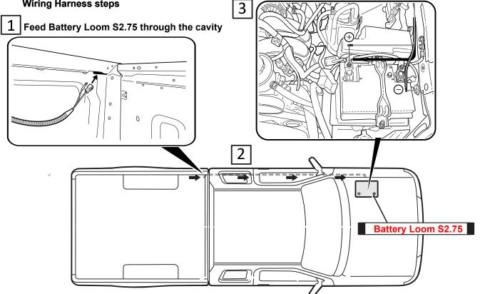
Run the wiring from the front corner cavity (leaving 200mm in the tub) to the battery over the chassis rail. Making sure to keep away from hot obstructions and cable tie every 400mm. Reconnect fuse patch to battery loom S2.75, now attach fuse patch to positive of battery and earth to the body of the Ute.
