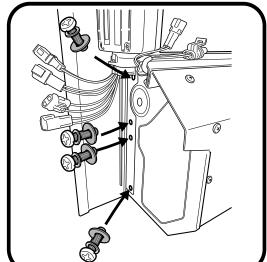
Connect motor connector to receiver
