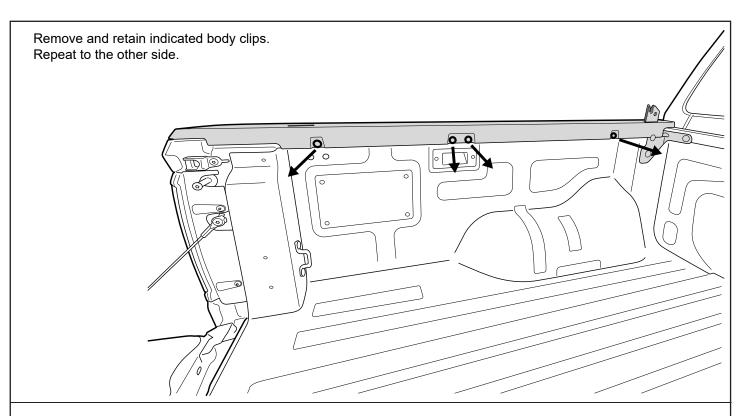
Carefully remove the plastic trim cap from the top of the tub, using assistance if necessary. Find the clip that holds the top trim of the tub and press the clips as needed to release the trim from the tub. Repeat to the other side.
