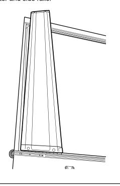
Using countersunk screws provided, line up end cap holes to the threads on the side rail.
